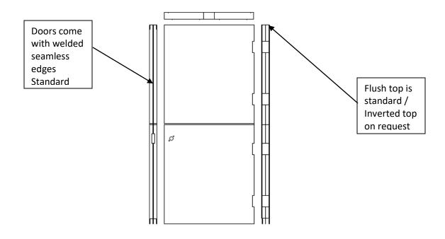
Polystyrene, Urethane, Honeycomb or Temperature Rise Core choices Your choice of door skin gauges and your choice of steel types: 18ga, 16ga, 14ga, 12ga or 10ga with CRS, A60, G90, or Stainless Steel # 304 or # 316
